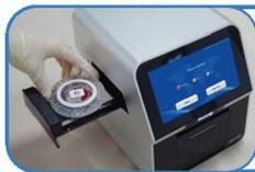
**02** Insert Disc (12-minute testing time )
