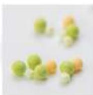
Precise freeze-dried beads to ensure the proper sample to chemistry ratio
